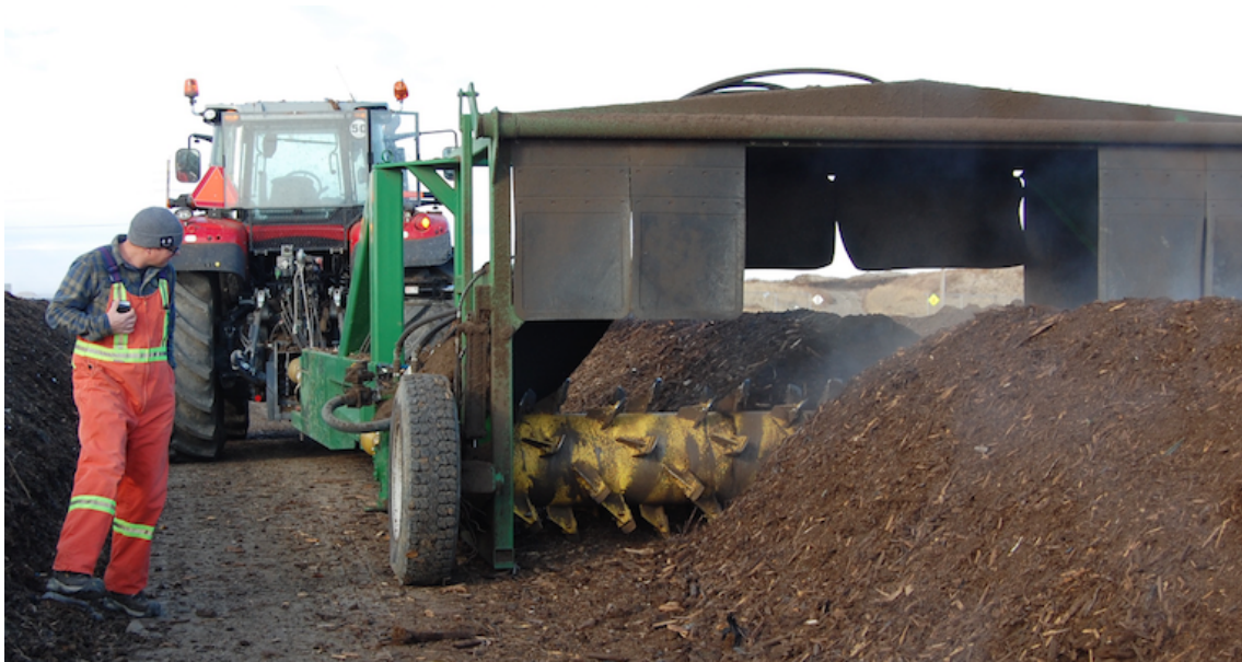
The operator checks the machine used to mix and pile the composting materials.
