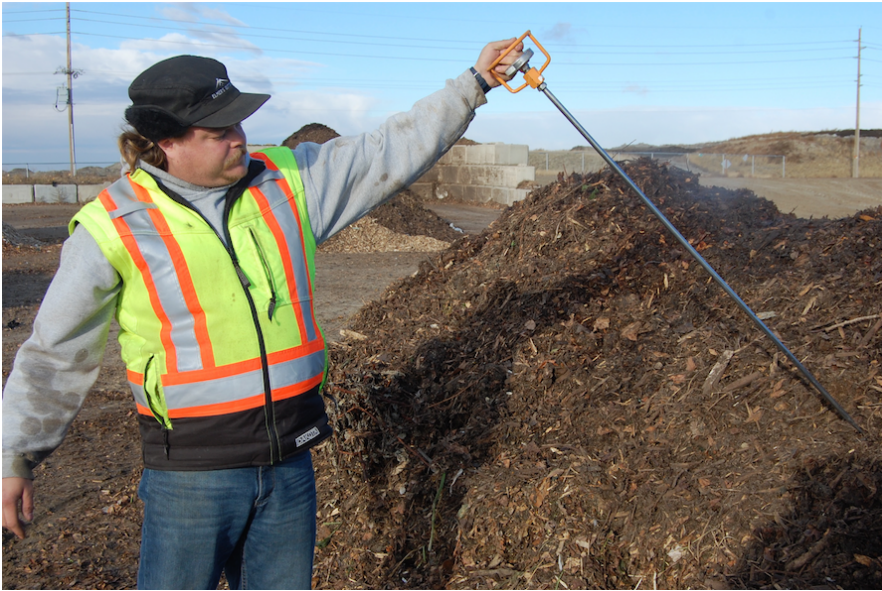
Riley taking the temperature of a steaming windrow.
